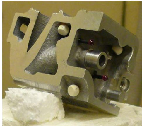
**Fig 13.** Setting of the BAM CT measurement 4011c with parameters 205 kV, filter 0.5 mm Cu + 0.75 mm Ag, 1800 angles, voxel size  $(50 \mu\text{m})^3$
