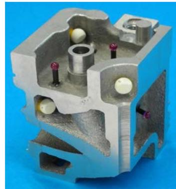
**Fig. 6.** Three mounted ZTA spheres on segment 1Al; ZTA 1 sphere is visible on bottom left
