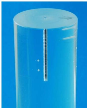
**Fig. 2.** PMMA cylinder with spherical landmarks [3], total size  $\varnothing 20 \text{ mm} \times 108 \text{ mm}$  (visible here top 30 mm), diameter of spherical landmarks 0.5 mm
