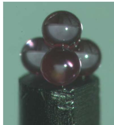
**Fig. 3.** Micro tetrahedron made from 4 ruby spheres of size 0.5 mm
