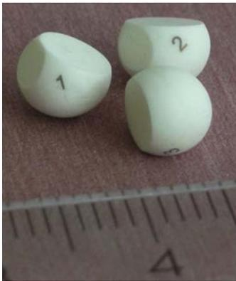
**Fig. 4.** ZTA (Zirconia Toughened Alumina) spheres with a diameter of 6.1 mm containing 86%  $\text{Al}_2\text{O}_3$  and 14%  $\text{ZrO}_2$
