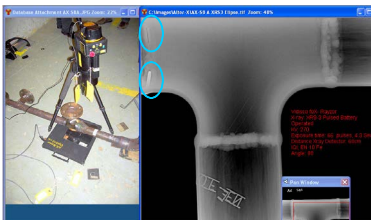
Figure 4. Set-up and Test X-ray of Carbon Steel 60mm Pipe
