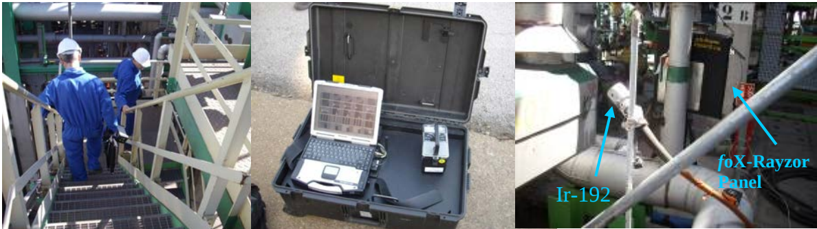
Figure 5. Working in the Refinery with the Portable DR System
