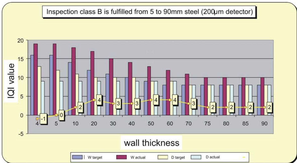
Figure 8. Compensation principle (3 steps) to achieve inspection class B
