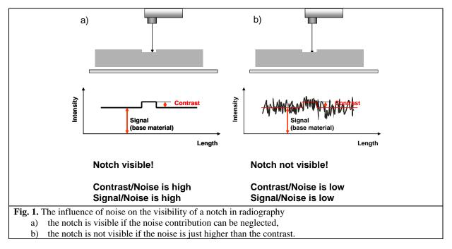
Now it is assumed that the hole diameter d is equal to the IQI thickness  $T = \Delta t$  (1T hole with  $d = T = \Delta t$ ). The just visible 1T hole diameter and IQI thickness can be calculated from eq. 2 and 3, if PT is known.
