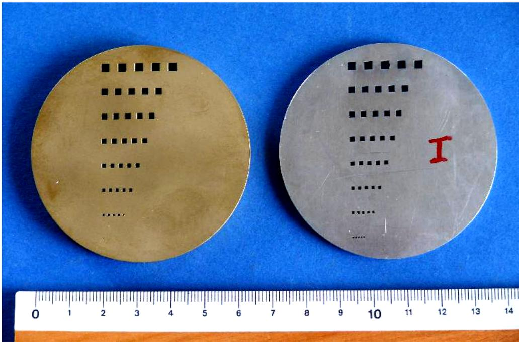
**Figure 4.** The test pieces machined at BAM, made of brass (left) and aluminium (right)
