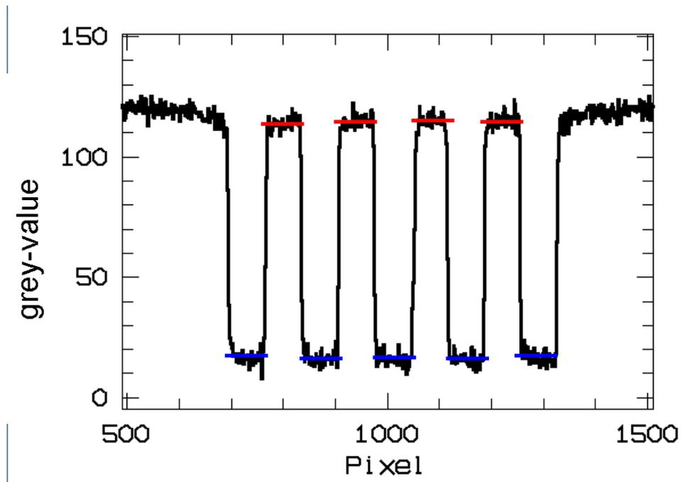
**Figure 9.** Determination of the minimum (blue) and maximum values (red) at an averaged line-profile from the measurement of the aluminium part
