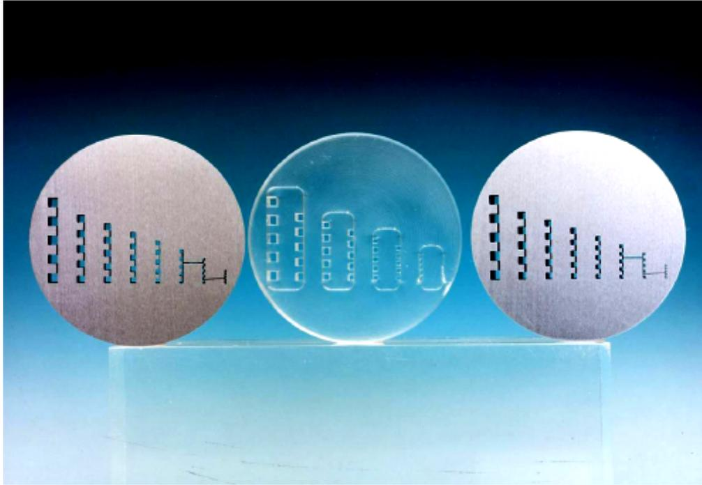
**Figure 2.** Test pieces with line-pair structures (from left to right: made of aluminium, acrylic glass, and steel; from FprEN 16016-3:2010)
