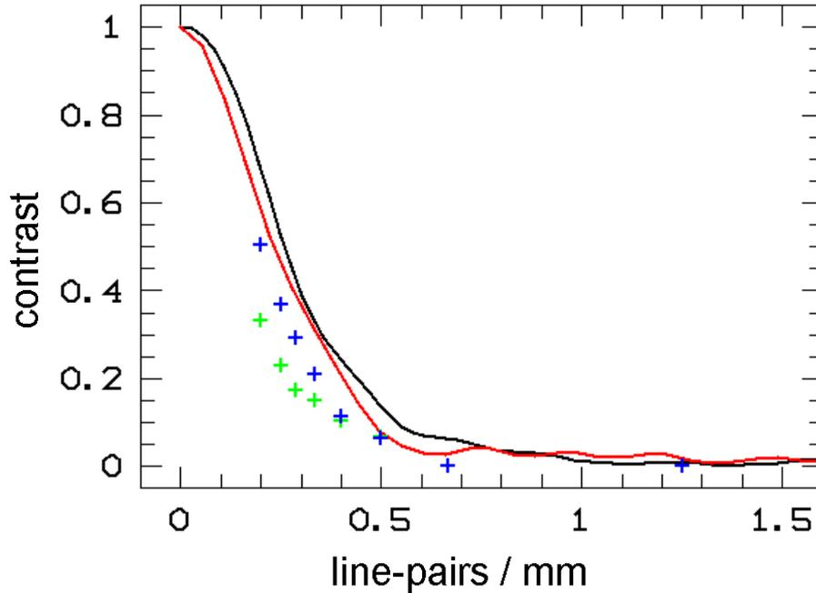
**Figure 7.** MTF determined at the brass test piece (black: without beam-hardening correction (BHC), red: with BHC) and contrast-factor  $R/100$  (blue: with BHC, green: without BHC)
