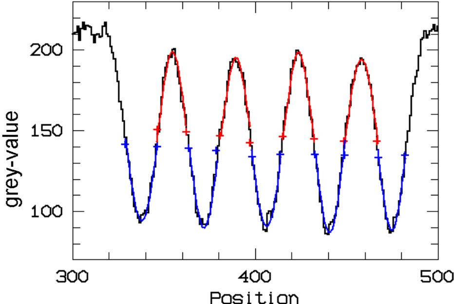
Figure 5. Gaussian curves fit to the maxima (red) and minima (blue) of an averaged line-profile
