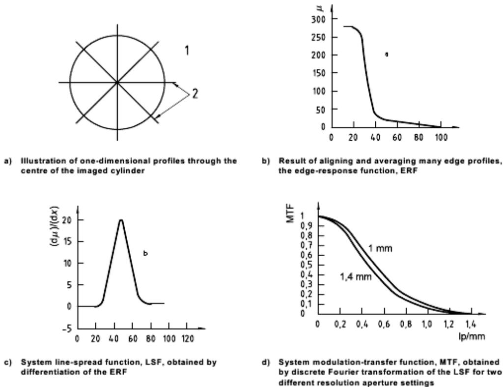
**Figure 1.** Determination of the MTF from the edge in the reconstructed CT data set of a cylinder (from ISO 15708-2:2002)
