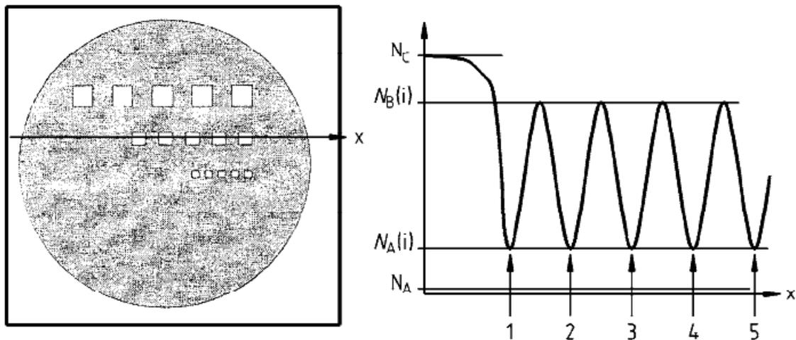
**Figure 3.** Determination of grey-value extrema at the line-pair structures (from FprEN 16016-3:2010)
