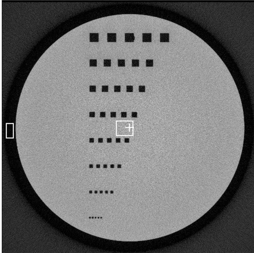
**Figure 8.** The reconstructed data set of the aluminium part with applied BHC. The centre of the fitted circle and the regions for determining the grey-values of the undisturbed material and the undisturbed background are indicated.
