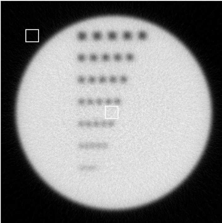
Figure 6. Location of the regions for determining the grey-values of the undisturbed material and background
