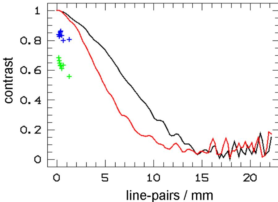
**Figure 10.** Results of the measurement of the spatial resolution at the aluminium part data set (black: MTF without BHC, red: MTF with BHC, blue: R/100 with BHC, green: R/100 without BHC)
