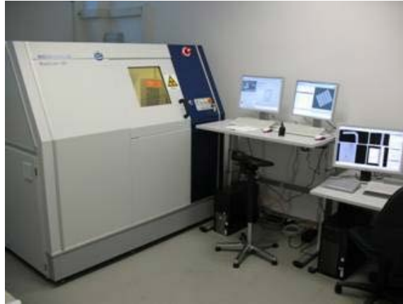
Figure 2. \mu -Computed Tomography system RayScan 150 from RayScanTechnologies at EADS Innovation Works
