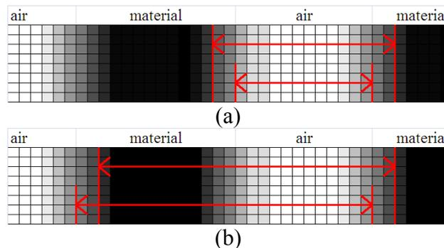
**Figure 2.** Edge dependent (a) and edge independent distances (b)
