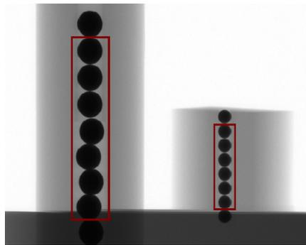
**Figure 5.** Test object with chrome steel spheres
