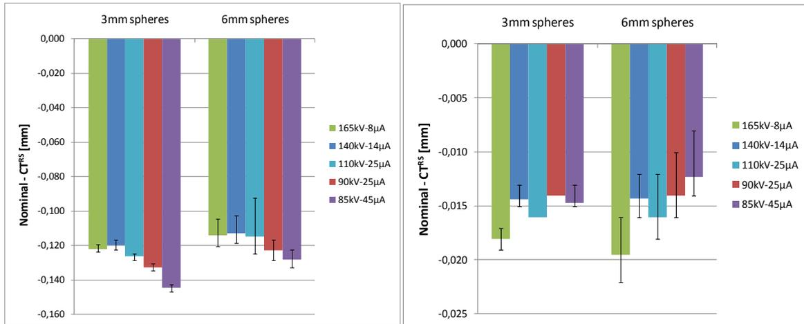
**Figure 6.** Deviations between the rescaled CT values and the nominal reference values of the sphere diameters for different voltage and current settings for global (left) as well as for local (right) thresholding
