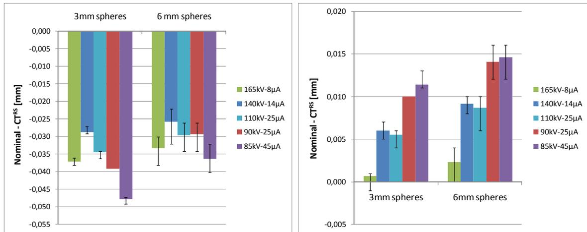
**Figure 7.** Deviations between the rescaled CT values and the nominal reference value of the sphere diameters for different voltage and current settings for global (left) as well as for local (right) thresholding, using a linear beam hardening correction method in the reconstruction step
