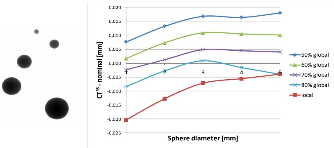
**Figure 8.** Left: Set-up with five chrome steel spheres with different sizes (diameters from 1 to 5 mm); Right: Deviations between rescaled CT values and the nominal value for spheres with different diameters measured with Varian 2520 detector
